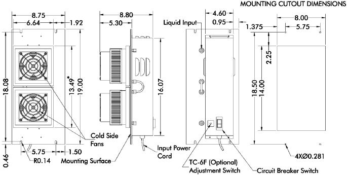
\* Dimension does not include hardware, insulation. Dimensions: inches.
